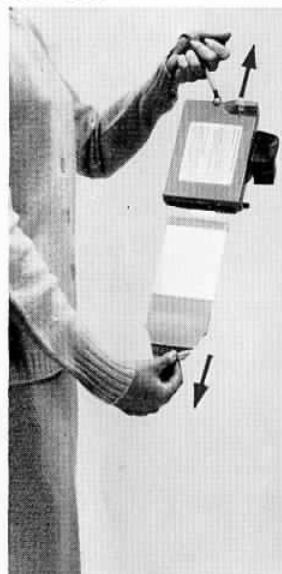
4. Pull the yellow tab all the way out of the camera: Pull it straight, smoothly, at medium speed, without slowing down or stopping.
